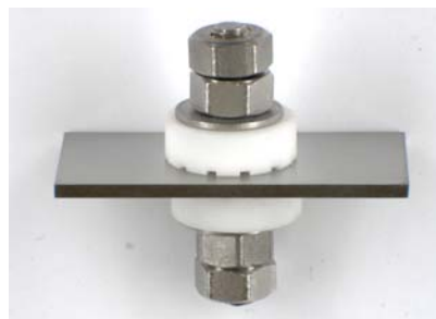
Figure 7: photography of a multi crevice assembly (MCA).
