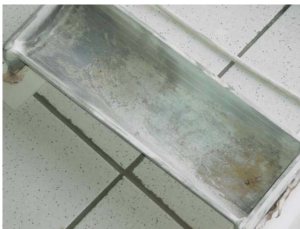
Figure 14: photograph of UNS S32304 sample after exposure in cell n°1
