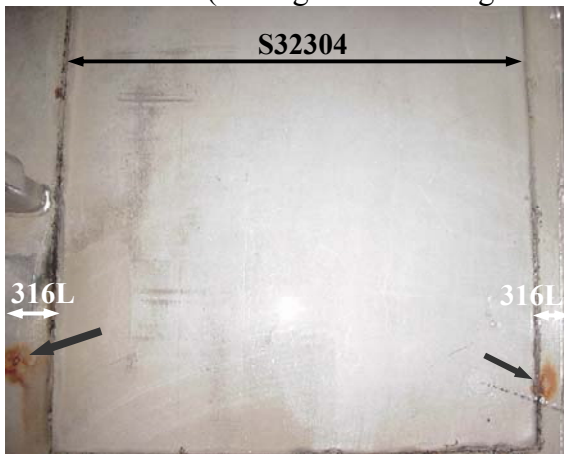
Figure 11: photograph of UNS S32304 welded onto 316L surface (arrows shows pitting attack)
