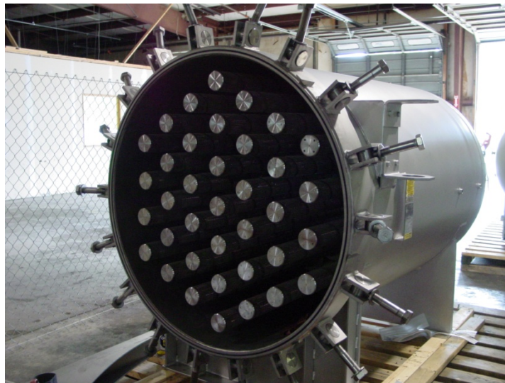
Figure 3 Filter Vessel constructed using AL-6XN Material
