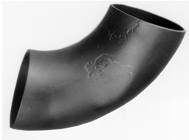
Figure 7 Long radius elbow showing surface pitting from catastrophic oxidation during improper annealing
